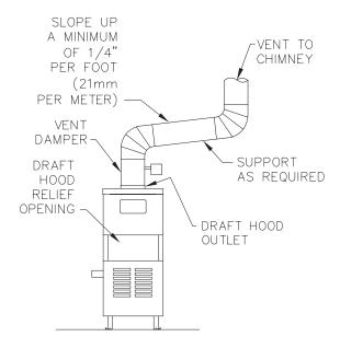
Figure 4.2: Venting with Vent Damper in Vertical Position
